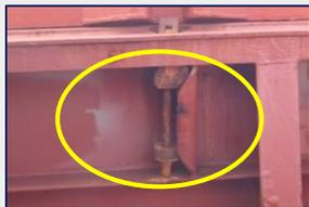
Whatever cleating system is used, it is of a paramount importance that it is structurally sound. Remember that cleats should never be overtightened to obtain a stiff seal. Excessive tightening makes the system too rigid resulting in cleat's damage.
