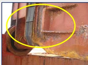
Packing rubber plays an important role in making hatch covers weathertight. A common practice is to use old rubber from shipboard stock, ignoring its exposure to the environment while idle or to mix new with old rubber. The rubber packing between hatch covers should be checked to ensure good condition, with a view to provide proper water tightness.
