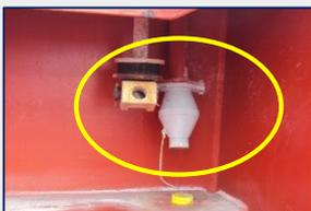
Drain system is the last safety barrier to water entry through the sealing system in a weathertight hatch cover system. If water enters the hatches, it will be collected in the drain channel and expelled through the drain pipe. Regular inspections and maintenance of the drain channels and pipes needs to be conducted to ensure their effective operation.
