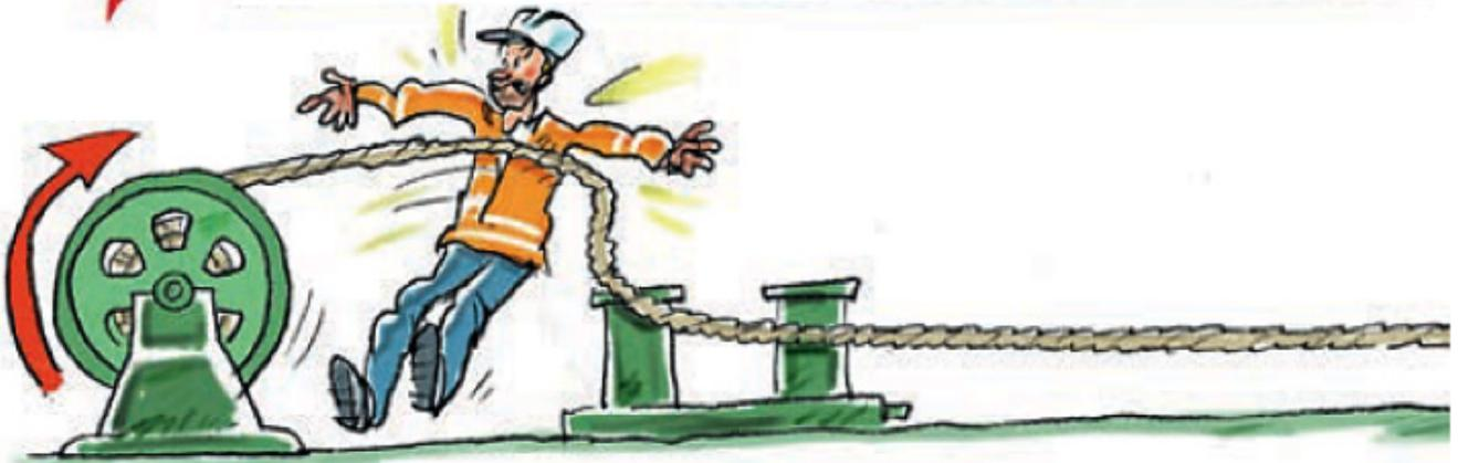
Line tension due to the weight of the line over side and the pull of the linesmen
