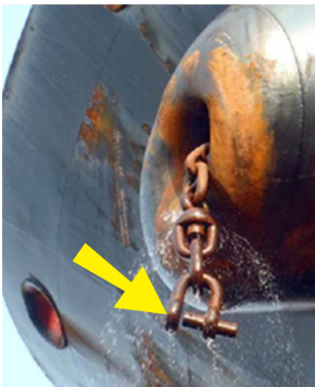
Photo – Anchor loss due to “D” shackle link opening up
